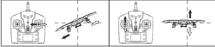
1. When moving throttle stick to left or right then the quadcopter is flying left or right at the same time.
