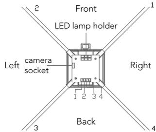
receipt board socket 1, connect with right-front electric wire
