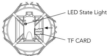
3. When Aerial is over, please disconnect the quadcopter and battery. Pull out the TF card, put the TF card into the reader, then connect the USB to computer. A few seconds later, you will find the Mobile hard disk from my computer and then you can see aerial data.
