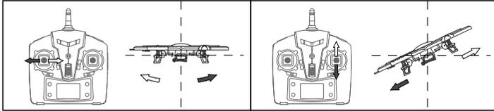
3. When moving forward and backward/ left and right flying stick to left or right, then the quadcopter is flying to left or right at the same time.
