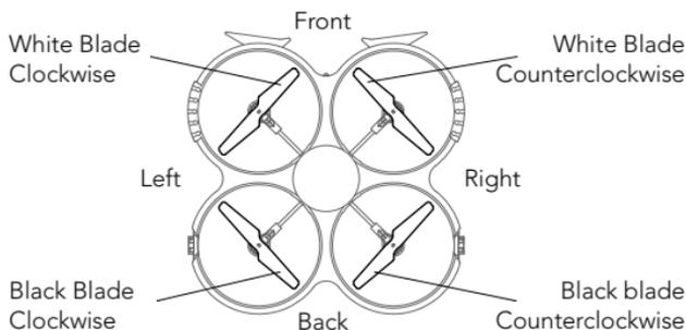
2. Power on the quadcopter check the rotating of blades. Left Front/Right rear blades rotating Clockwise, Right front/Left behind rotating Counterclockwise.
